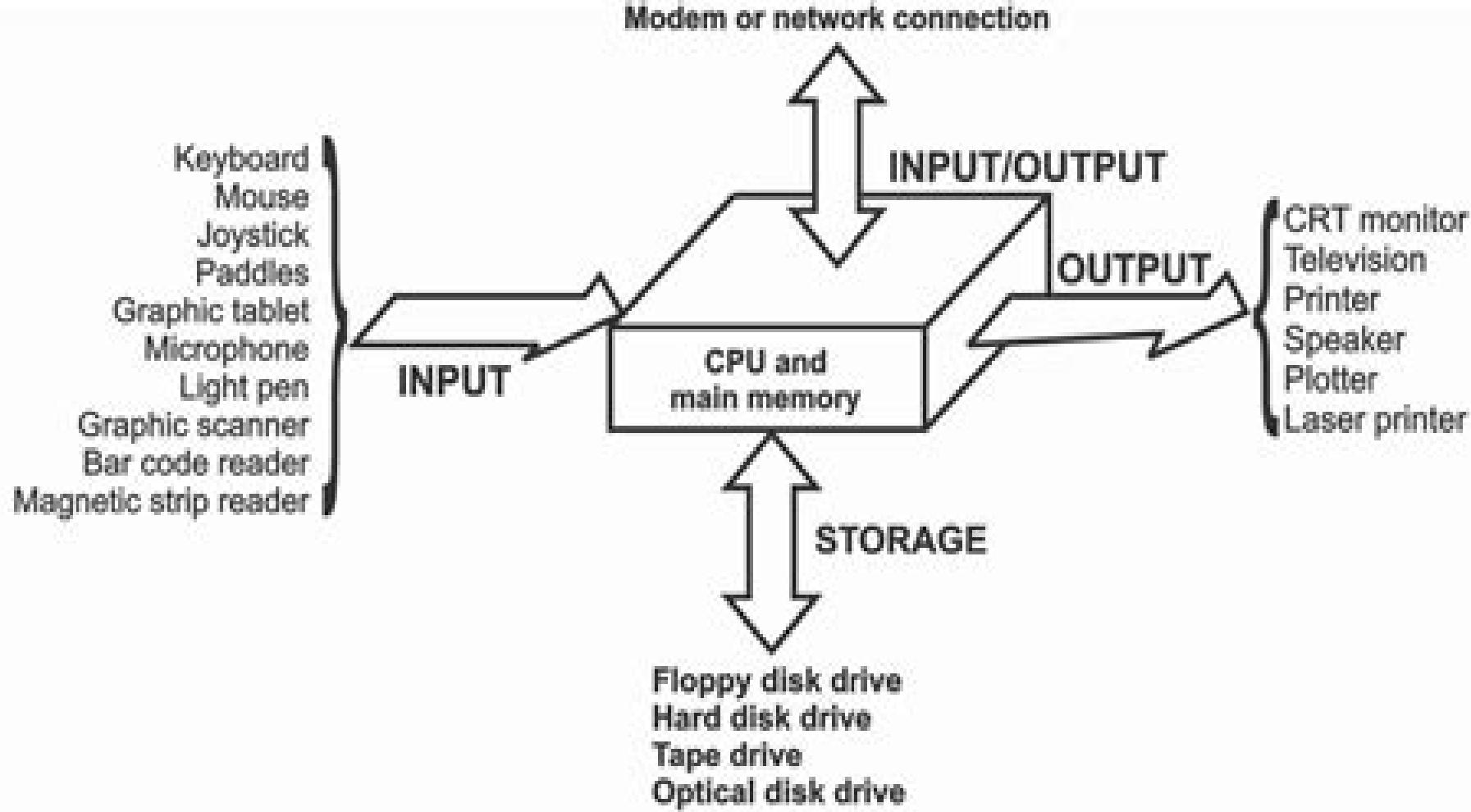
**Fig 11.8 Peripheral devices commonly attached to the CPU of a microcomputer.**
