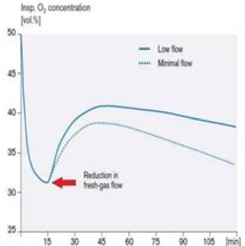
To maintain inspiratory oxygen concentration during low flow anaesthesia increase fresh gas O<sub>2</sub> conc by 50%
