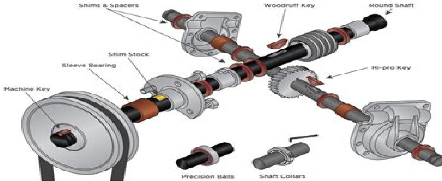
**Mechanical Power Transmission** is the transfer of energy from its source to another location using mechanical elements.
