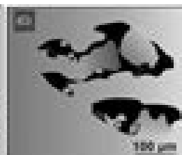
Lack of fusion (incomplete or partial melting)
