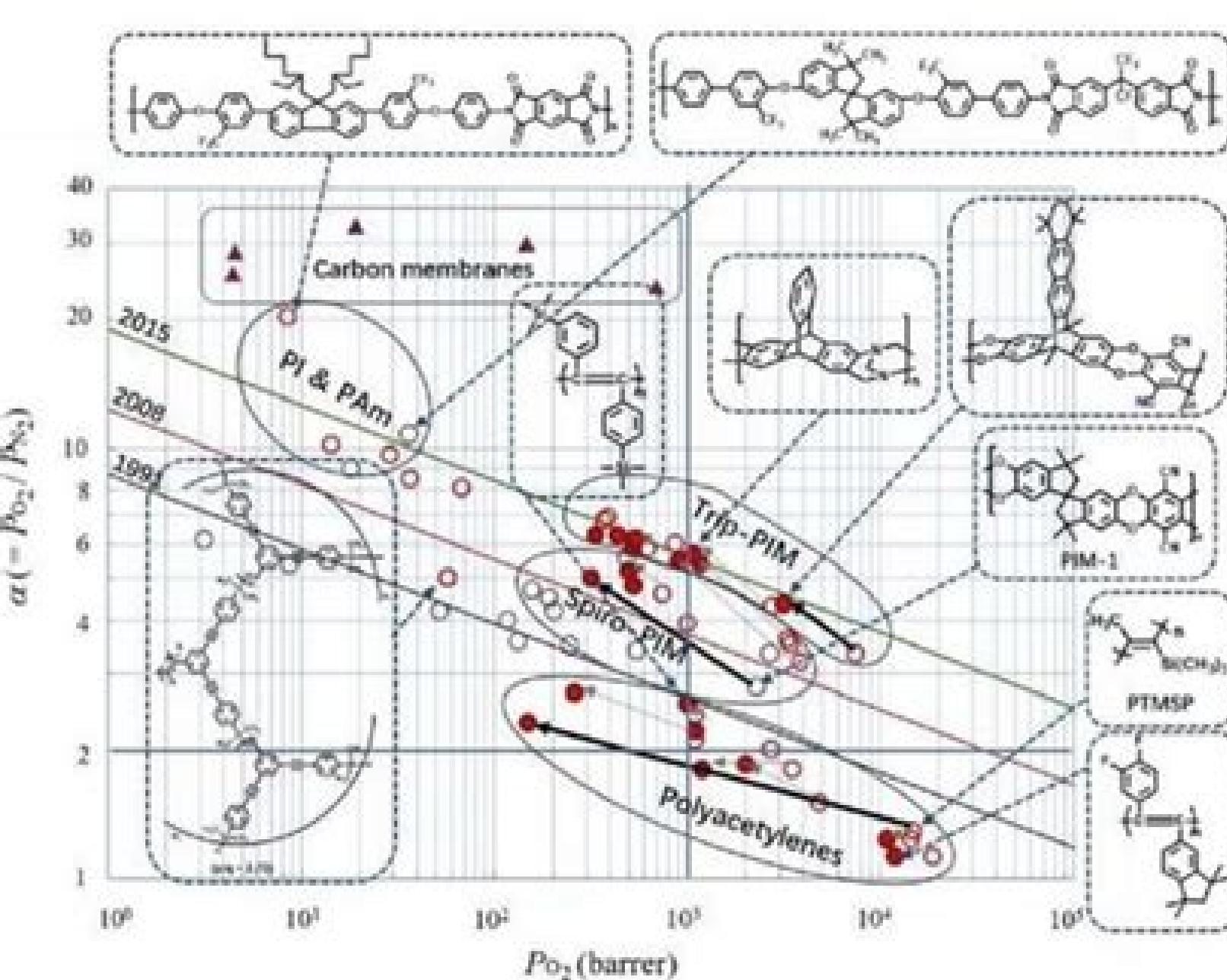
Upper plots through polymers showing the highest  $\alpha$  at each  $P_{O_2}$  reported in the literature in 2020 (●: after aging, ○: before aging).
