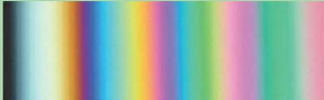
Photograph of a quartz wedge between cross-polarizers rotated 45° from extinction showing the different orders of retardation colors increasing from left to right. These colors are a true representation and not those typically seen in "colored" Michel-Levy color charts. As such, these form the background image for the retardation chart from Dyar and Gunter (2020). *Photograph courtesy of Mickey Gunter of University of Idaho.*
