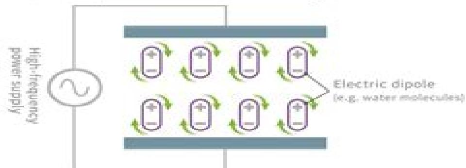
When a high-frequency electrical field is applied, the water molecules (electric dipoles) flip with each alternating electrical field, and heat is generated by friction.
