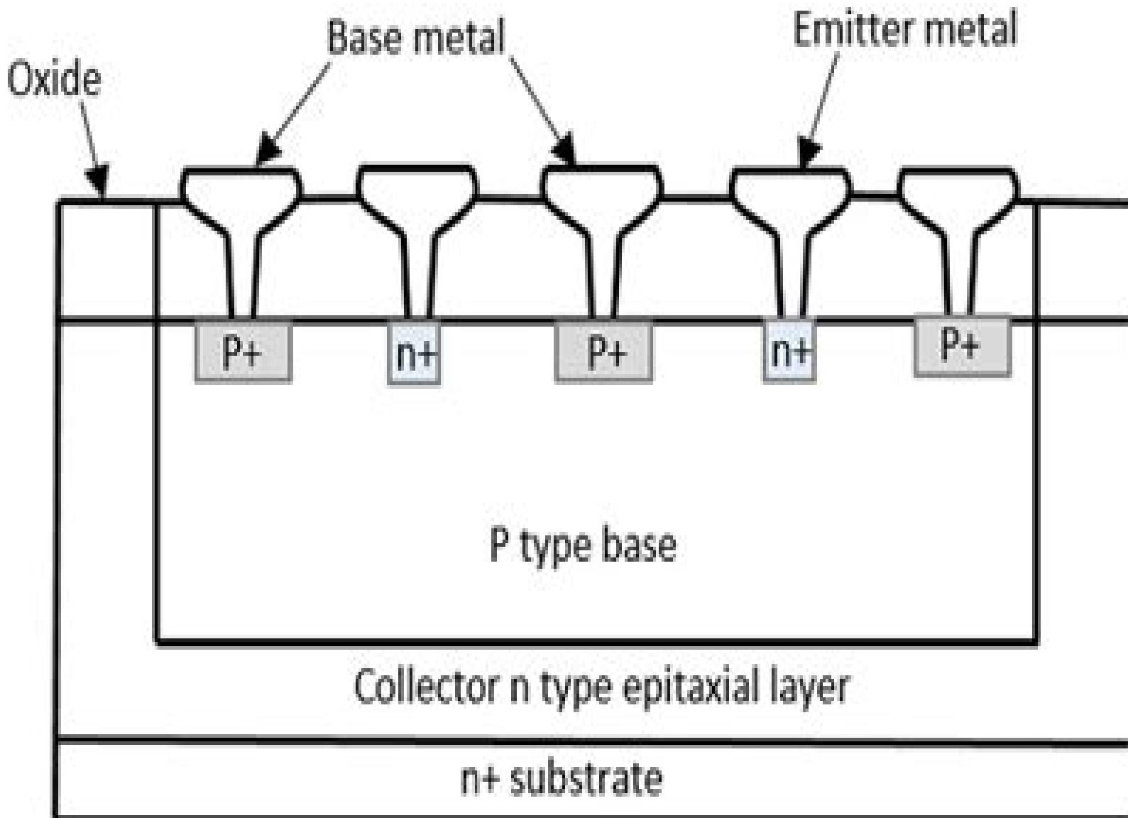
n-p-n silicon double diffused epitaxial transistor
