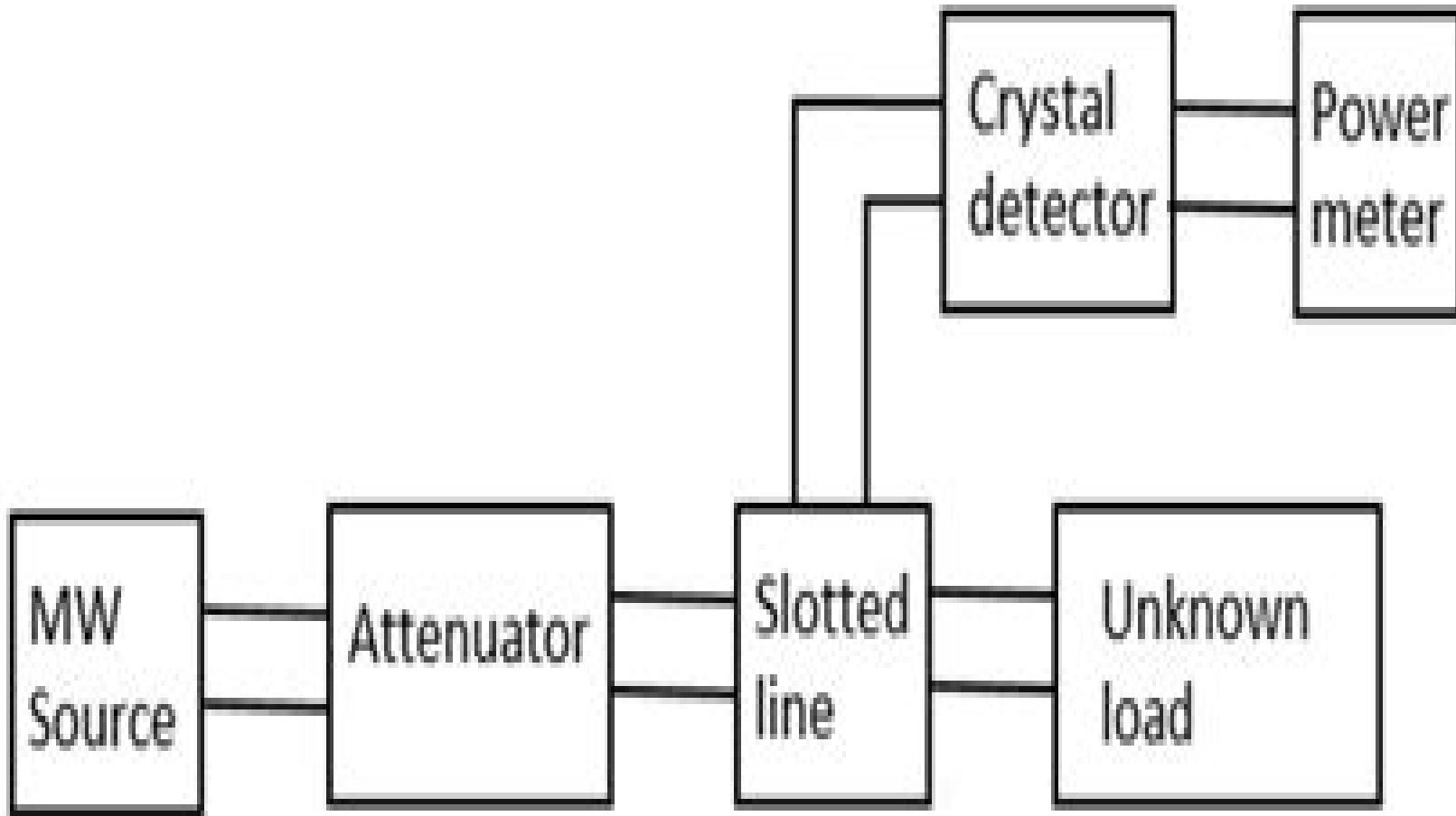
Set up 1, Impedance measurement using slotted line
