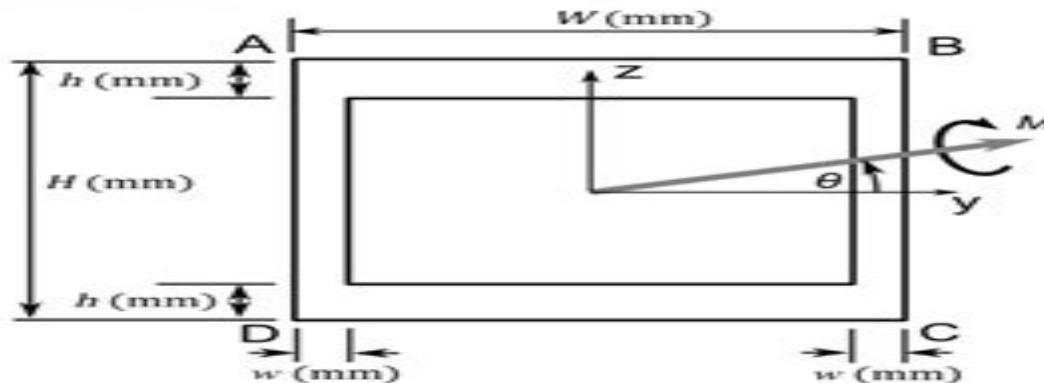
A hollow box beam (cross section depicted in the figure, not to scale) is made of a material of Young's modulus  $E$ .
