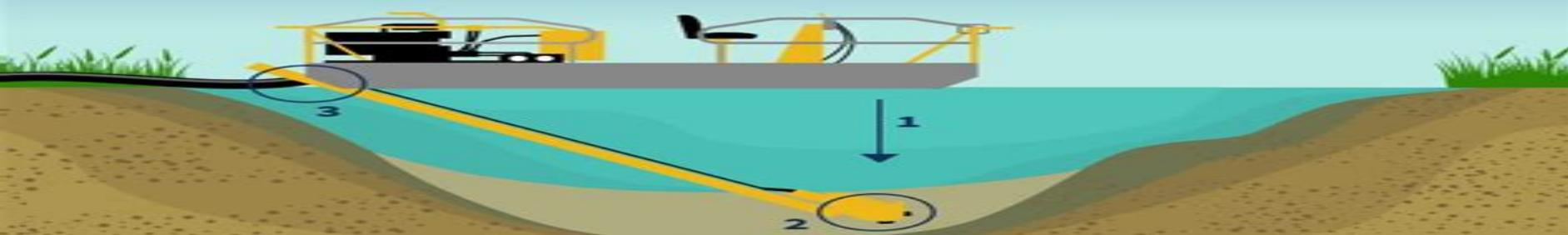
**1** The operator of the dredge **lowers the boom** to the bottom of the body of water.
