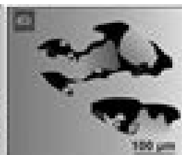
Lack of fusion (incomplete or partial melting)
