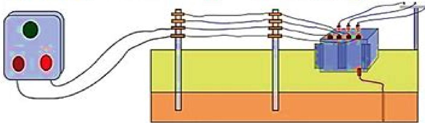
The neutral grounding is nothing but connecting the neutral point of the supply system or rotating machine or transformer to the earth directly or through some circuit elements. A three-phase system can be operated in two ways, they are ungrounded or isolated neutral system and grounded or earthed neutral system (i.e., neutral grounding).
