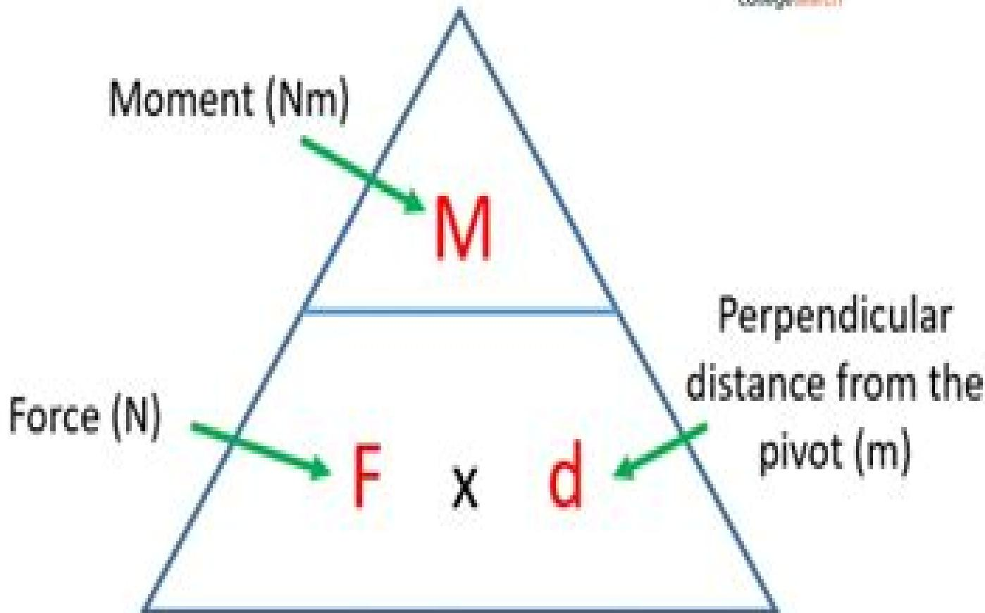
$$\text{Moment (Nm)} = \text{Force (N)} \times \text{Distance (m)}$$
