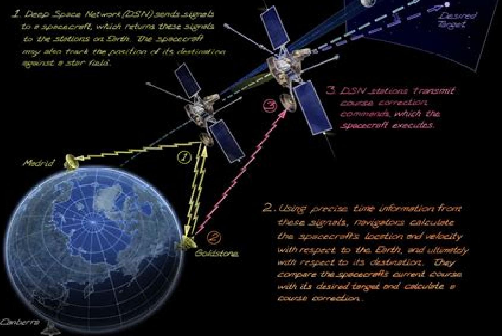
2. Using precise time information from these signals, navigators calculate the spacecraft's location and velocity with respect to the Earth, and ultimately with respect to its destination. They compare the spacecraft's current course with its desired target and calculate a course correction.
